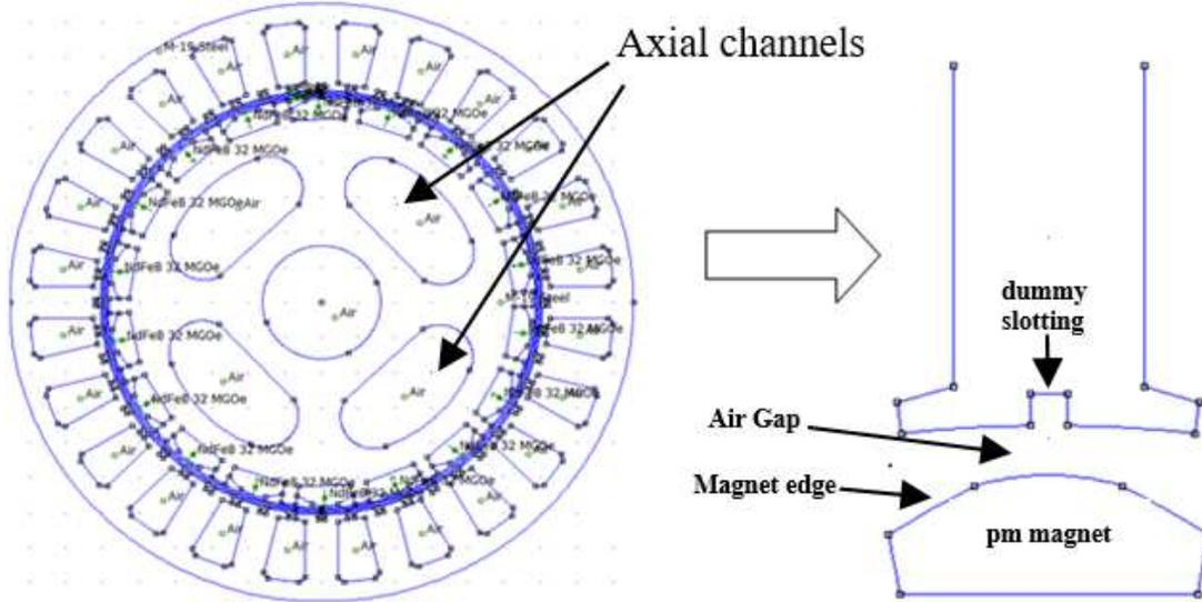
Fig. 2 PMG of proposed structure
