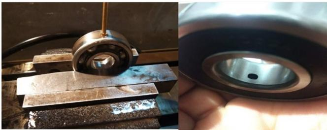
Fig. 5 Inner race and outer race faults simulation
