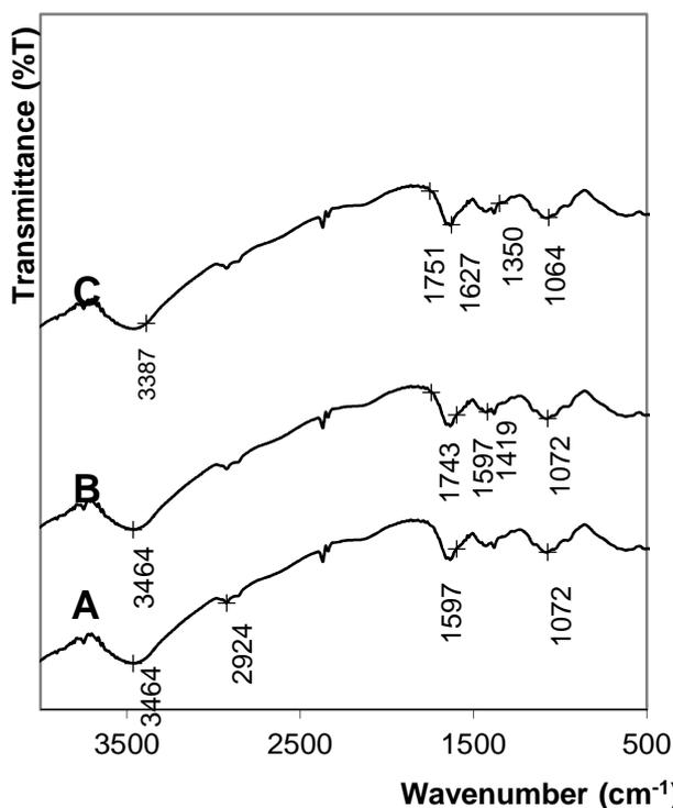
Fig. 11 FTIR test result from membrane: A. Chitosan; B. Pectin; C. Pectin-Chitosan-BADGE
