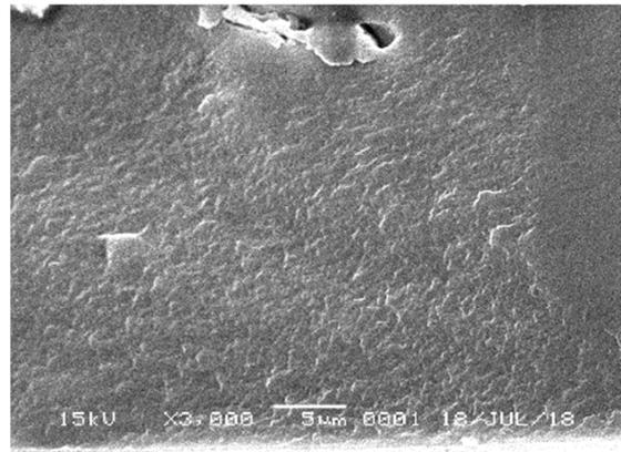
Fig. 9 SEM test result of a cross-section from membrane chitosan
