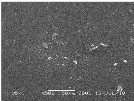
Fig. 6 SEM test result of the surface from membrane chitosan
