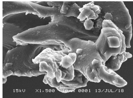
Fig. 10 SEM test result of a cross-section from membrane Pec-Chi-BADGE
