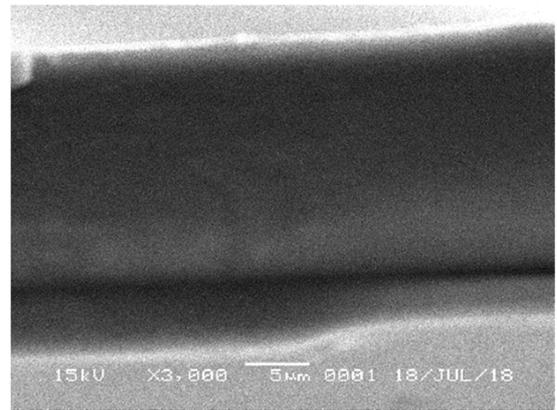
Fig. 8 SEM test result of a cross-section from membrane pectin
