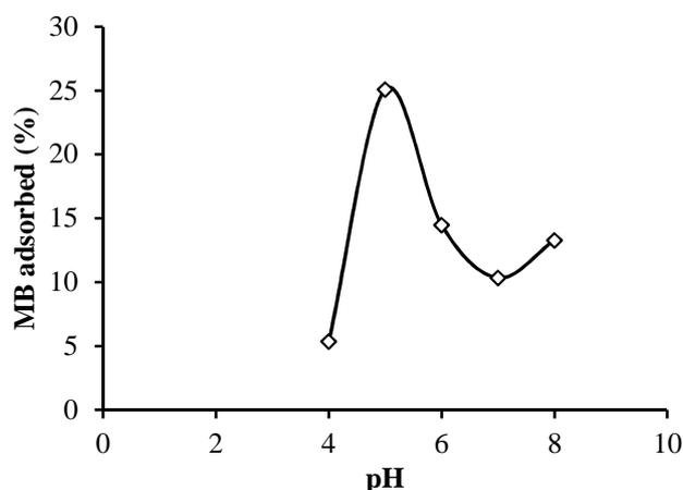
Fig. 12 The methylene blue adsorption by Pec-Chi-BADGE membrane
