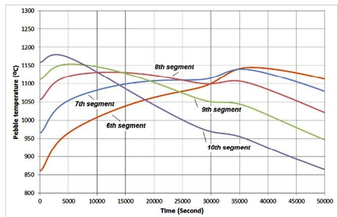
Fig. 6 Transient of pebble temperature (5 lowest segments) in the middle core following the event with the insertion of FTC
