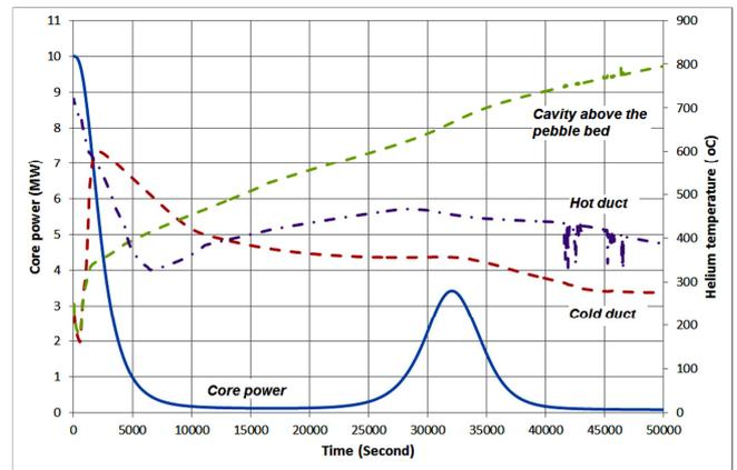
Fig. 5 Transients of the core power and helium temperature in the primary system
