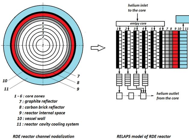
Fig. 2 Developed core model and core heat loss using RELAP5
