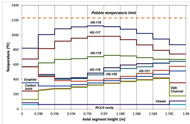
Fig. 7 The temperature of the pebble in the core, graphite and carbon brick reflector, reactor internal space, vessel, and air in the RCCS cavity
