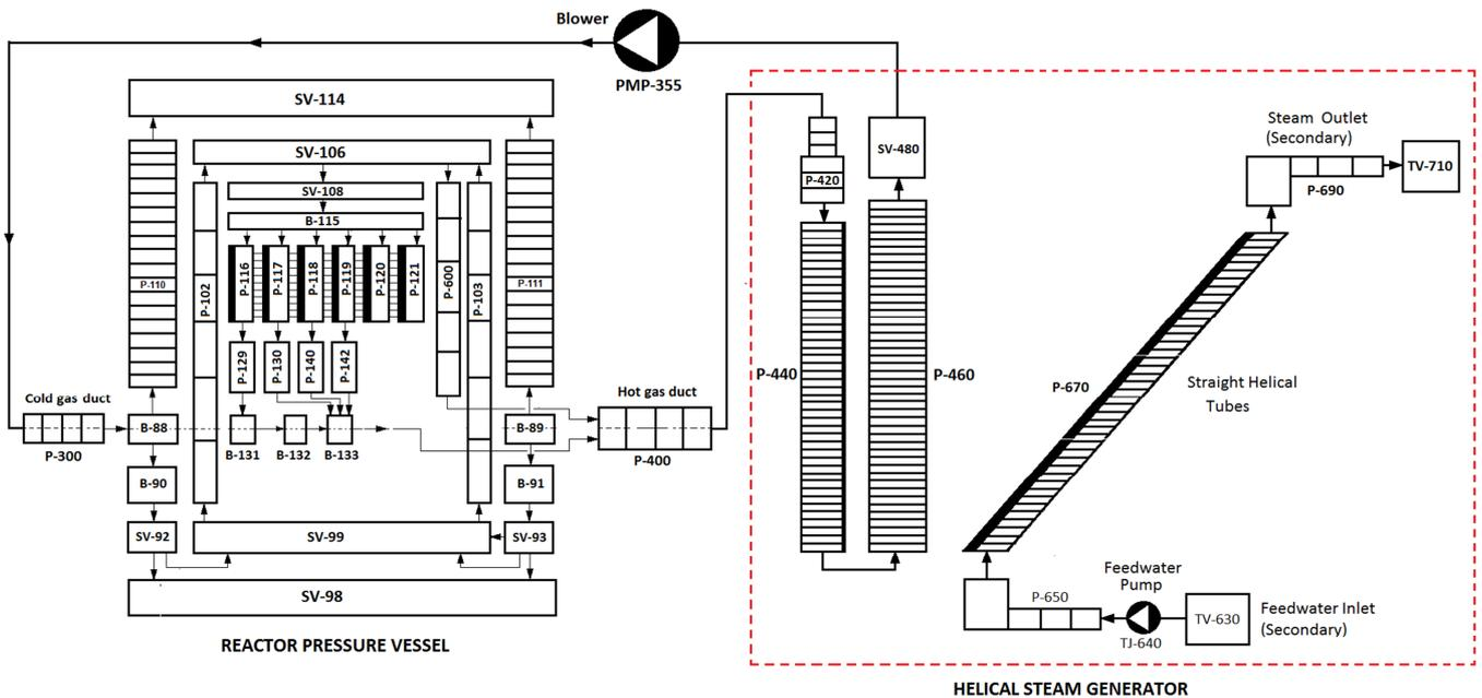
Fig. 3 The integrated model of RDE Nuclear Steam Supply System (NSSS) developed by RELAP5 code
