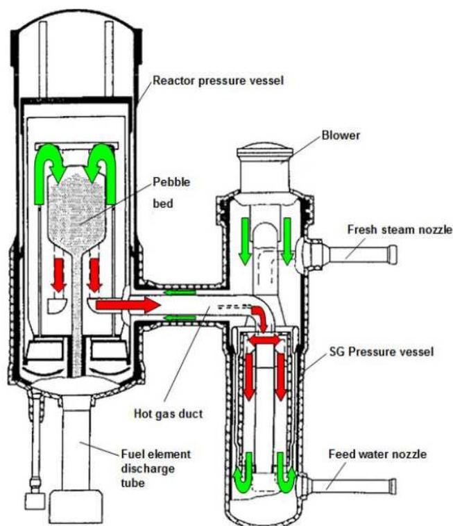
Fig. 1 Main components of the RDE and the helium flow path inside
