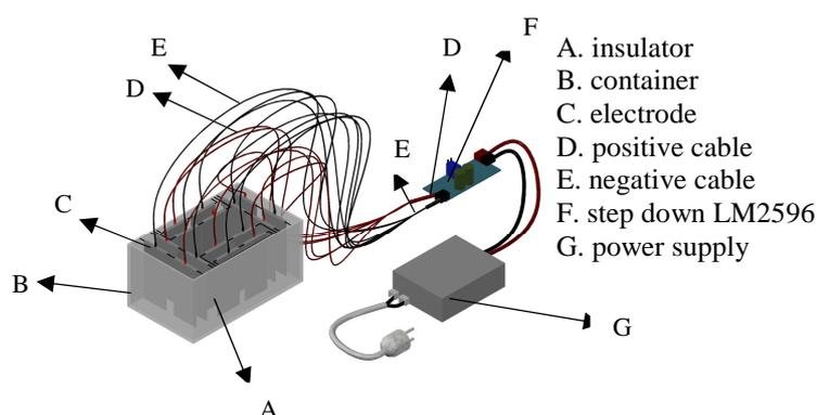
Fig. 1. Electrocoagulation design
