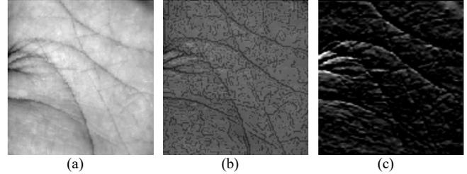
Fig. 6 Edge detection process, (a) Contrast stretching image (b) Canny image (c) Sobel image
