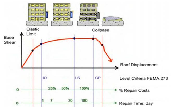
Fig. 2 Capacity curve of the building
