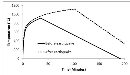
Fig. 5 Comparison of the parametric fire curve before and after an earthquake [11]
