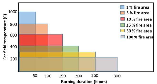
Fig. 7 Travelling fire curve [33]
