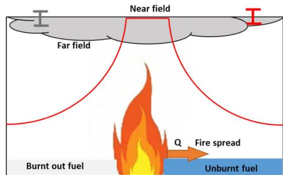
Fig. 6 The concept of travelling fire [35]
