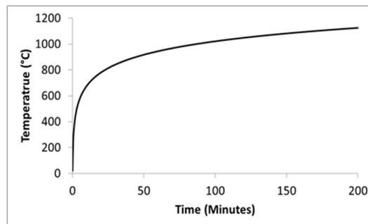
Fig. 3 ISO 834 Standard fire curve [27]
