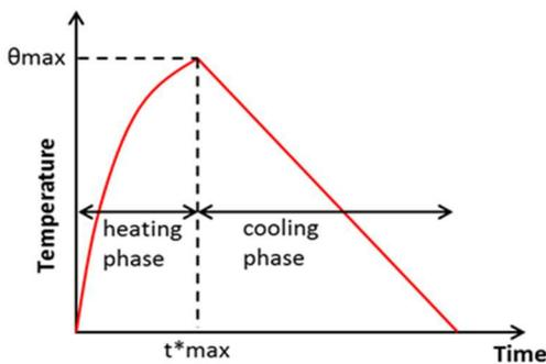
Fig. 4 Eurocode parametric fire curve [32]
