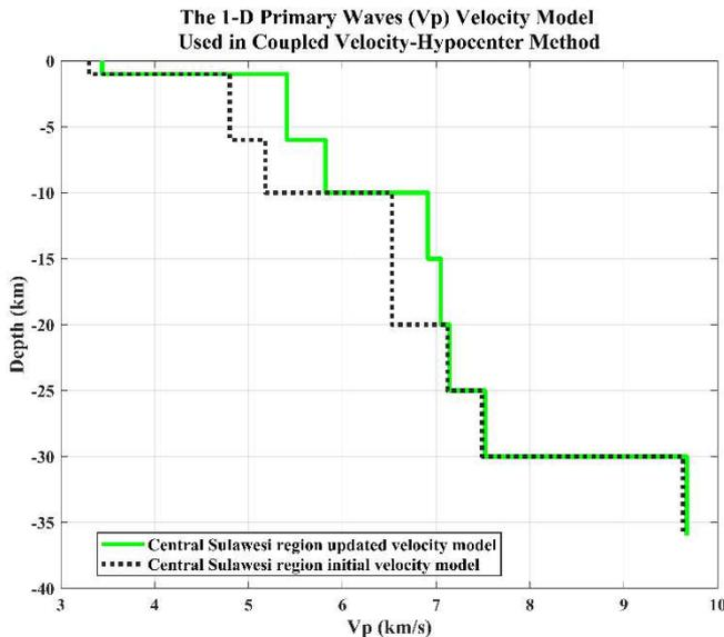
Fig. 7 The Central Sulawesi 1-D Primary waves ( $V_p$ ) velocity model used in Coupled Velocity-Hypocenter Method
