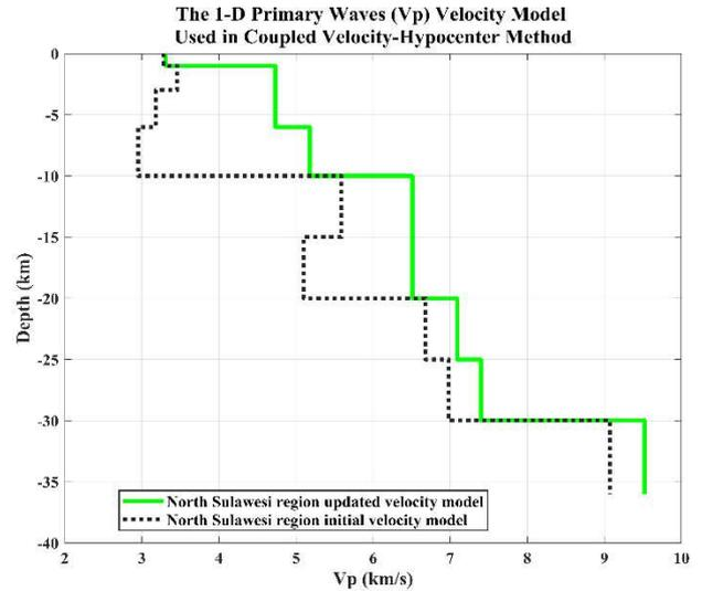
Fig. 6 The North Sulawesi 1-D Primary waves (Vp) velocity model used in Coupled Velocity-Hypocenter Method
