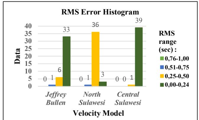
Fig. 4 RMS error residual histogram of relocation result using different velocity models.
