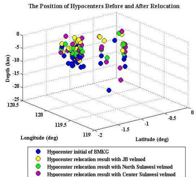
Fig. 2 Location of hypocenter before relocation and hypocenter after relocation by Coupled Velocity-Hypocenter method using three different velocity models.
