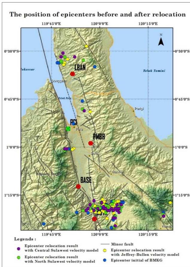
Fig. 3 Initial epicenters location and location of the epicenters after being relocated by Coupled Velocity-Hypocenter method using three different velocity models
