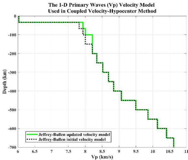
Fig. 5 The Jeffrey-Bullen 1-D Primary waves (Vp) velocity model used in Coupled Velocity-Hypocenter Method
