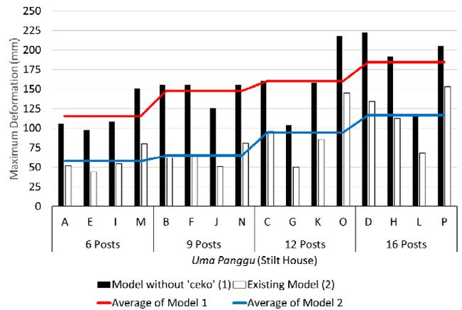
Fig. 8 Comparison of the maximum deformation (mm) between the models without diagonal bars (*ceko*) and existing models in each type of stage house (*uma panggung*)
