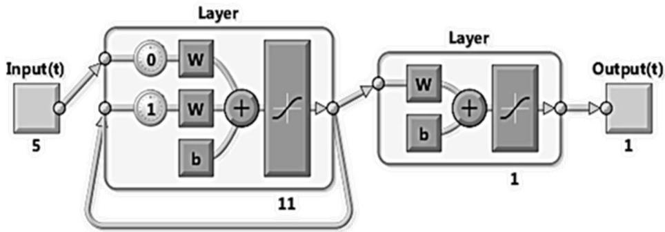
Fig. 2 The structure of RNN
