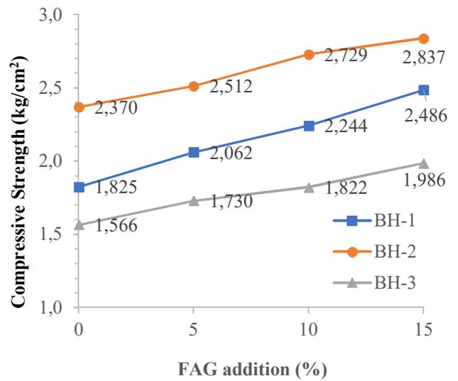
Fig. 5 The compressive strength of natural soils under study at different FAG addition
