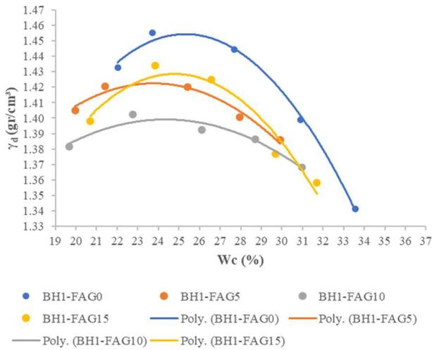
Fig. 1 Compaction Curve of BH1 soil at different FAG additions
