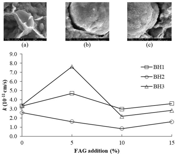
Fig. 6 The permeability and SEM images of natural soils in the study at (a) 5% wt. (b) 10% wt. and (c) 15% of FAG addition
