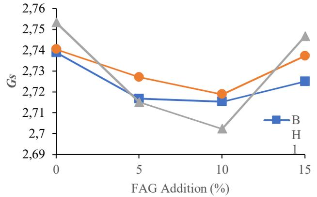
Fig. 4 The specific gravity of natural soils under study at different FAG addition
