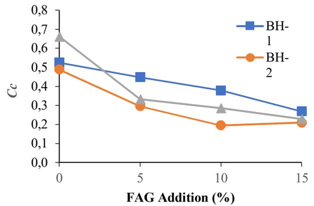
Fig. 10 The compression index of natural soils under study at different FAG addition
