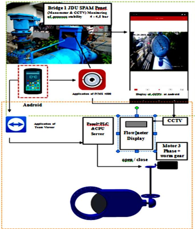
Fig. 3 Process flow of automatic valve design
