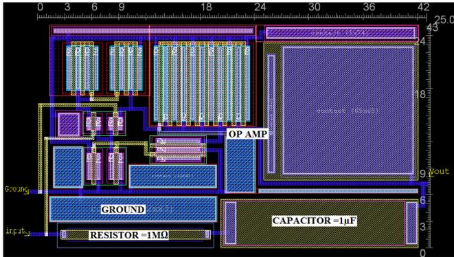
Fig. 7: Monolithic Integrator layout
