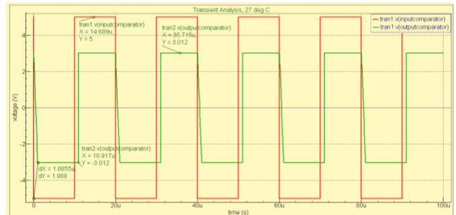
Fig. 5 Output of comparator
