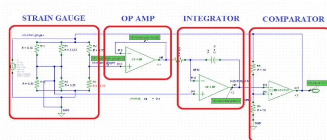
Fig. 1 Schematic of SFC
