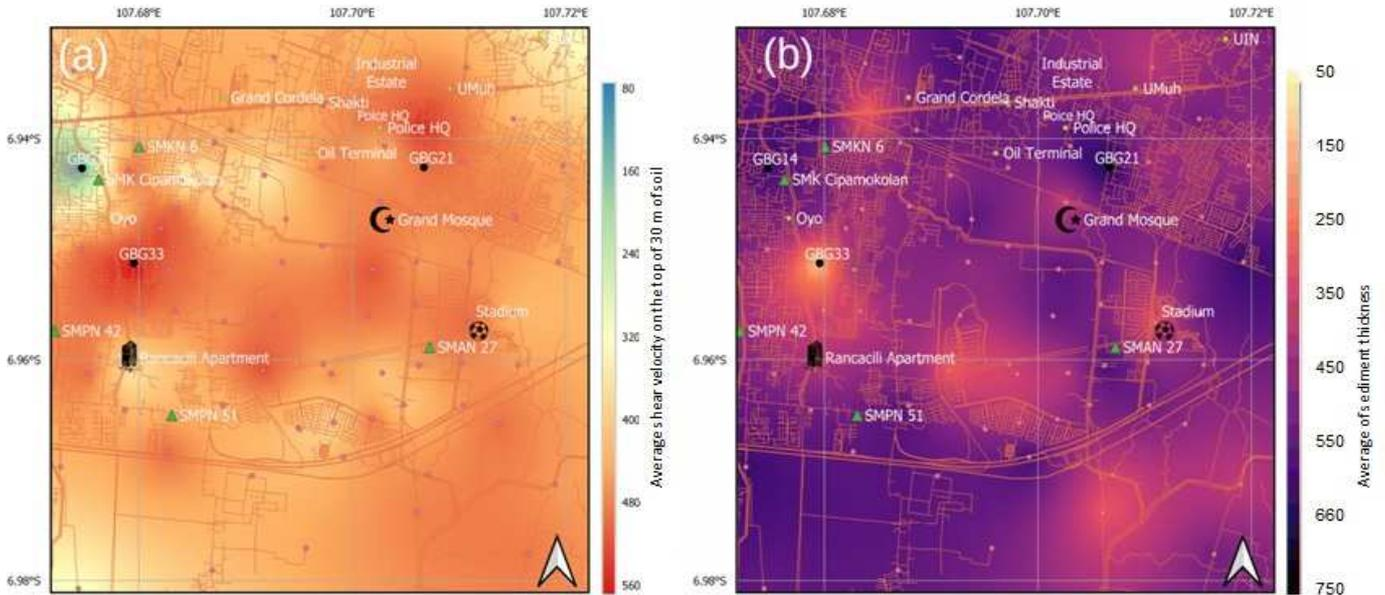
Fig. 6 Maps of (a)  $V_{s30}$  and (b) sediment thickness (Z1.0) inferred from the inverted shear-wave velocity of Gedebage area. Figure 6a show the variation value of  $V_{s30}$  in the study area between 80 m/s and 560 m/s and dominated by the value of  $V_{s30}$  from 320 to 480. Only a small area has a value of 160 m/s and value of 560 m/s. Figure 6b show sediment thickness of study area ranging from 50 to 750 m.
