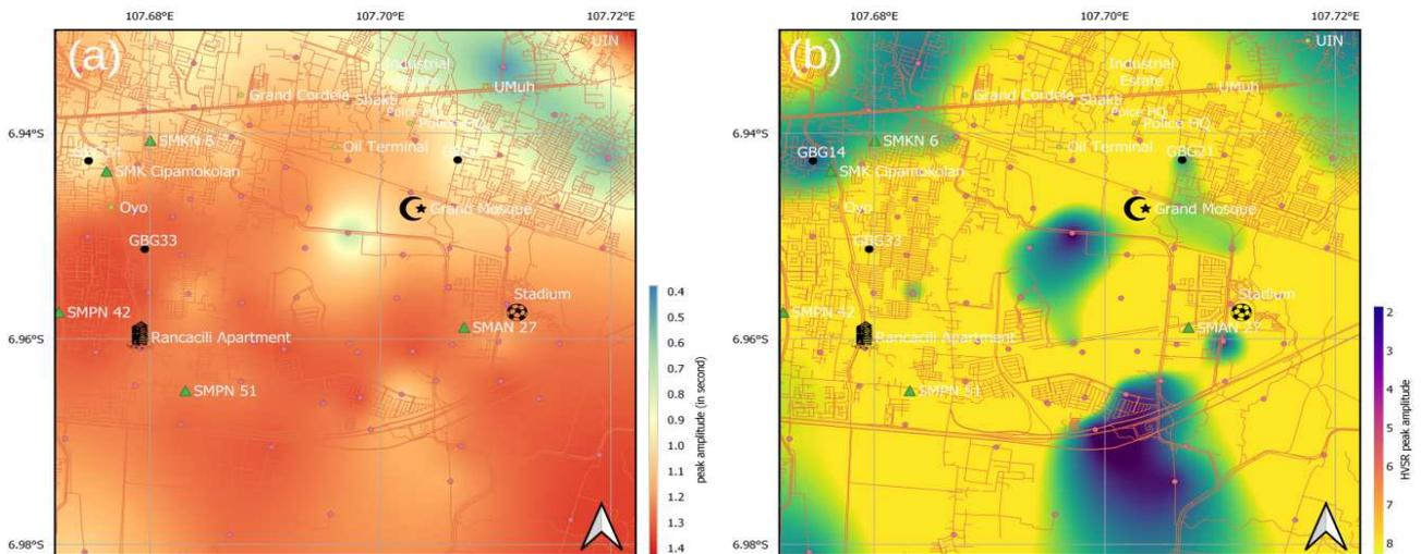
Fig. 4 Maps of HVSR (4a) peak period and (4b) peak amplitude. The figure 4a shows that peak period from 0.4 to 1.4 second mean medium and soft rock, mainly in the range of 1.2 – 1.4 second. Figure 4b shows the peak amplitude of the study area that mostly in the range 7 – 8; they reach lower in some areas.
