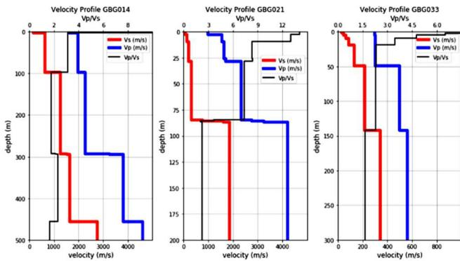
Fig. 5 The velocity profile for three sampling location with different depth.
