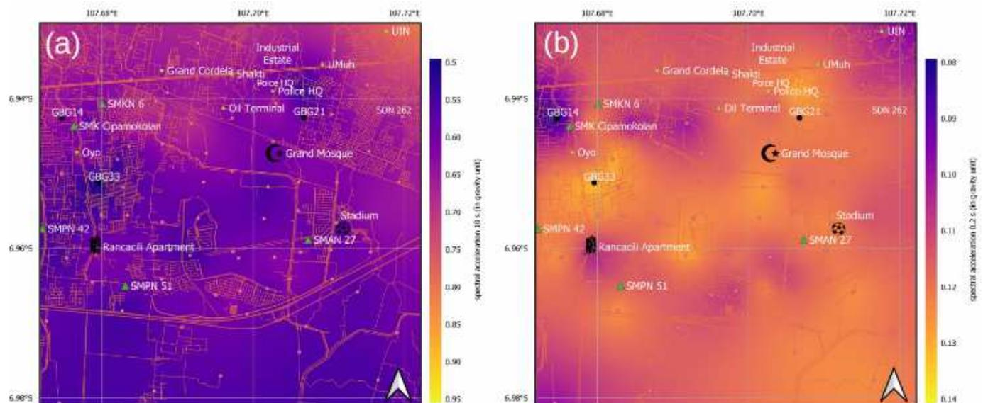
Fig. 7 Maps showing spectral acceleration for period 0.2 second (SA:0.2) resulted from scenarios (a) Mw6.8 event generated by Lembang Fault and (b) a megathrust event with a magnitude of Mw8.7. Notes: for a clearer view, these figures using different scale bars.
