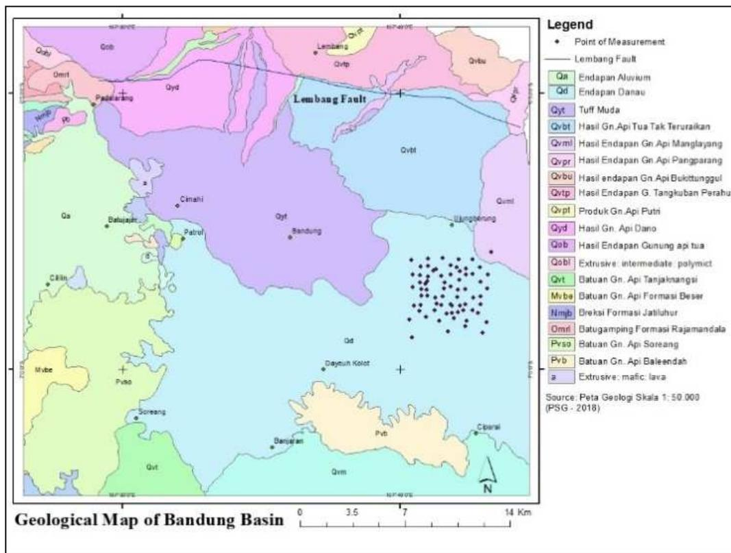
Fig. 3 Geology map of the Bandung basin is compiled and simplified from previously published maps [14]-[17]. The picture also shows the measurement location of microtremor (black dots).
