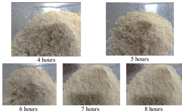
Fig. 2 Corncoobs Powder with Different Drying Durations
