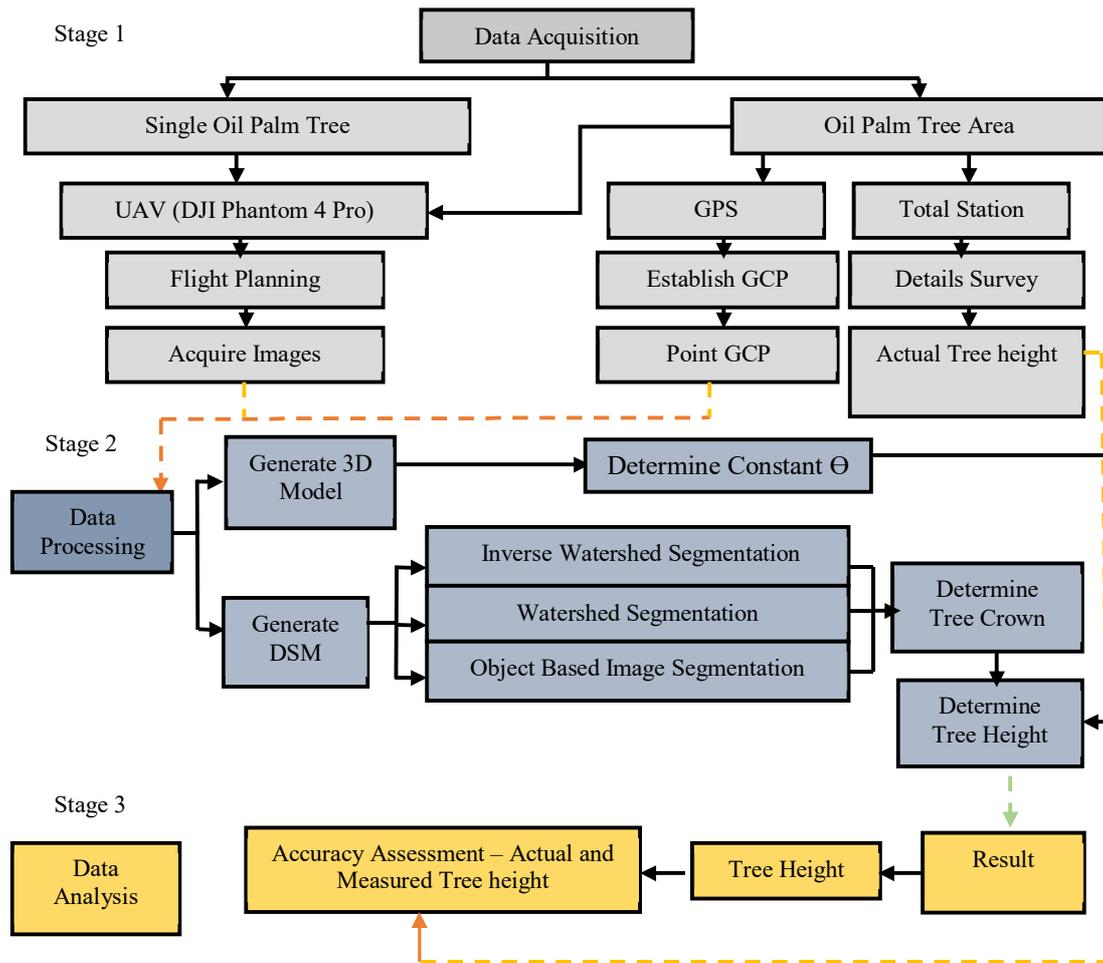
Fig. 1 Research Methodology in Determination Tree Height using UAV Images
