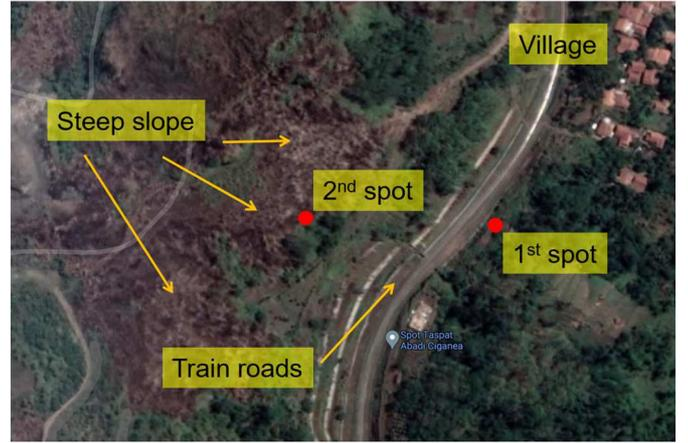
Fig. 7 Location of extensometer installation in the prone landslide area facing a double-track train road.
