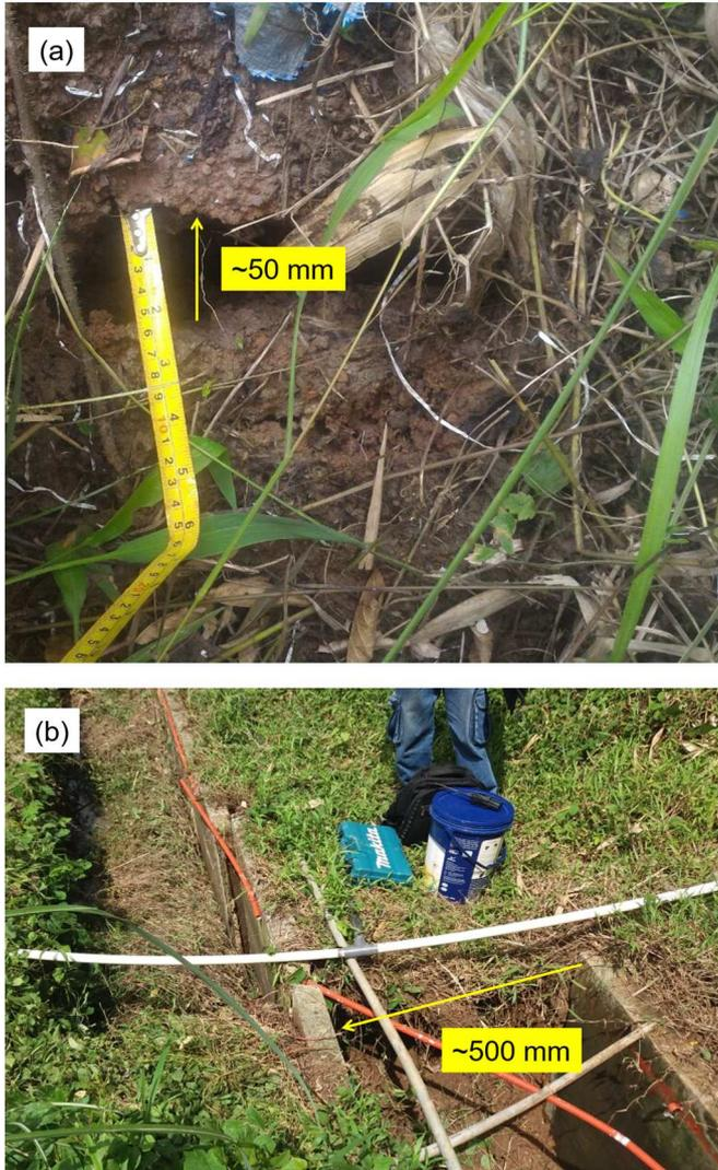
Fig. 11 Actual investigation on the measurement spot showing soil shift of  $\sim 50$  mm and  $\sim 500$  mm at the 1<sup>st</sup>-spot and the 2<sup>nd</sup>-spot, respectively.
