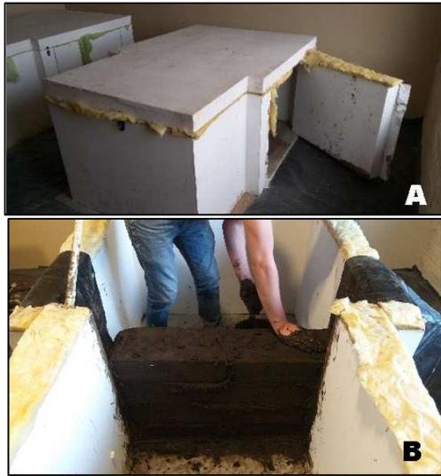
Fig. 5 (A) Acoustic and thermal test chamber, (B) Adobe block wall inside the test chamber
