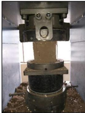
Fig. 2 Compressive strength test of adobe block
