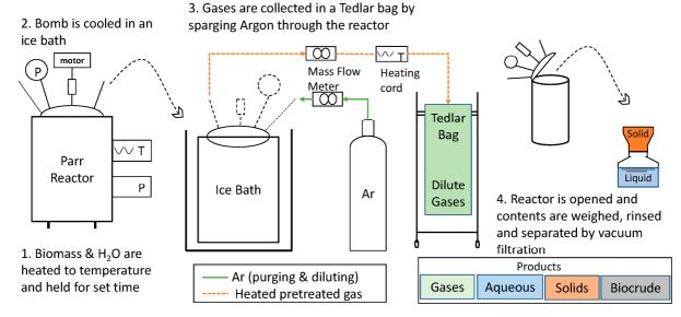
Fig. 5 HTL flow process [141]
