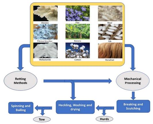
Fig. 8 The fiber extraction flowchart from biomass [194]
