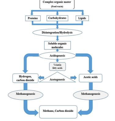
Fig. 7 Different phases in the anaerobic digestion process [154]
