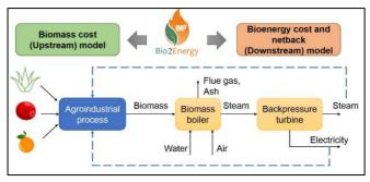
Fig. 2 Overview of biomass application for energy [51]
