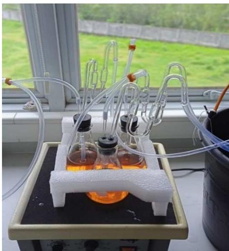
Fig. 1 Cocoa Pod Husk Bioethanol Fermentation Bioreactor
