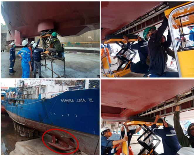
Fig. 2 Gondola mounting Construction on RV Baruna Jaya III
