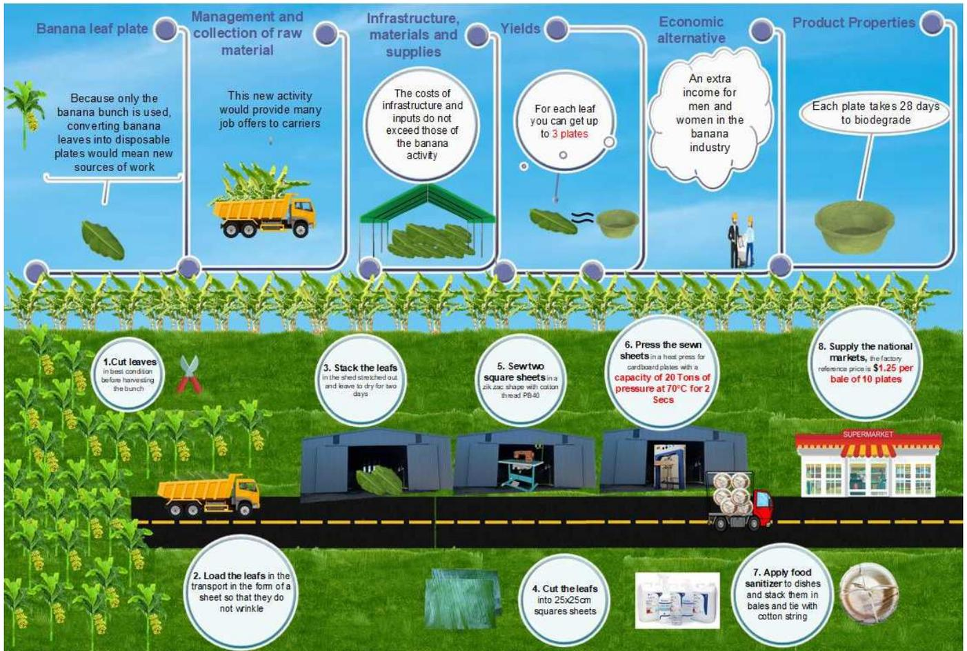
Fig. 5 Infographic for the process of elaboration of disposable plates made from banana leaves. The high-resolution image can be found and downloaded on the following link: [https://figshare.com/articles/figure/Infographic\\_Banana\\_leaf\\_plates/20819911](https://figshare.com/articles/figure/Infographic_Banana_leaf_plates/20819911)
