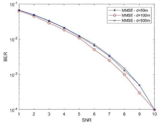
Fig. 10 BER performance of MMSE at different Tx-Rx distances
