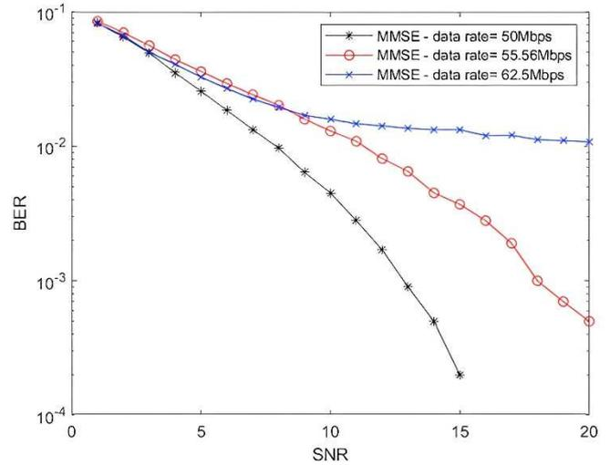
Fig. 14 BER performance of MMSE simulated under NLOS at different data rates
