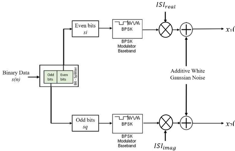
Fig. 5 Block diagram of a transmitter
