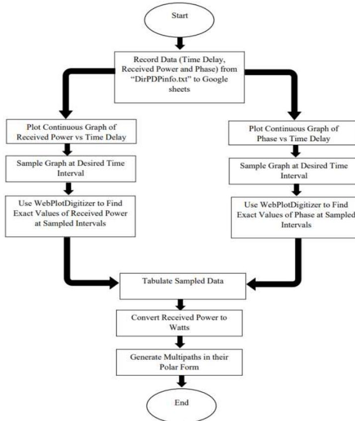
Fig. 2 Block diagram of sampling process
