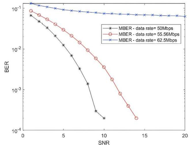
Fig. 11 BER performance of MBER simulated under LOS at different data rates
