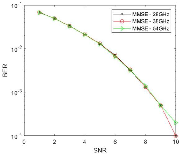
Fig. 8 BER performance of MMSE at different frequencies
