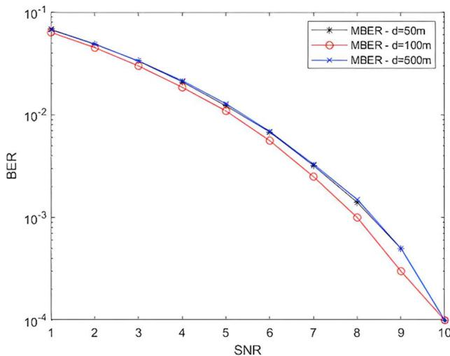
Fig. 9 BER performance of MBER at different Tx-Rx distances
