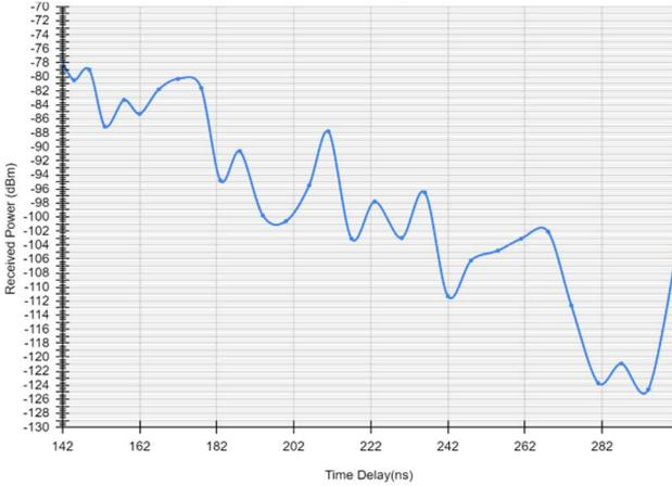
Fig. 3 Sampling of received power at 20ns interval
