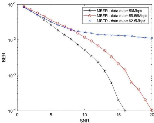
Fig. 13 BER performance of MBER simulated under NLOS at different data rates
