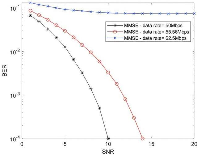
Fig. 12 BER performance of MMSE simulated under LOS at different data rates
