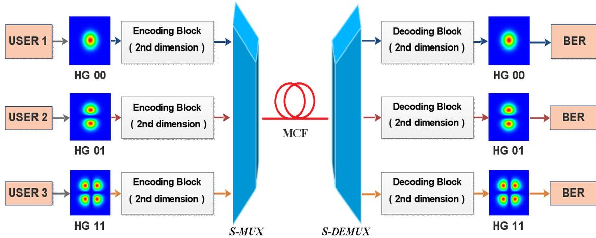
Fig. 3 OCDMA system architecture based on HG mode and MCF.
