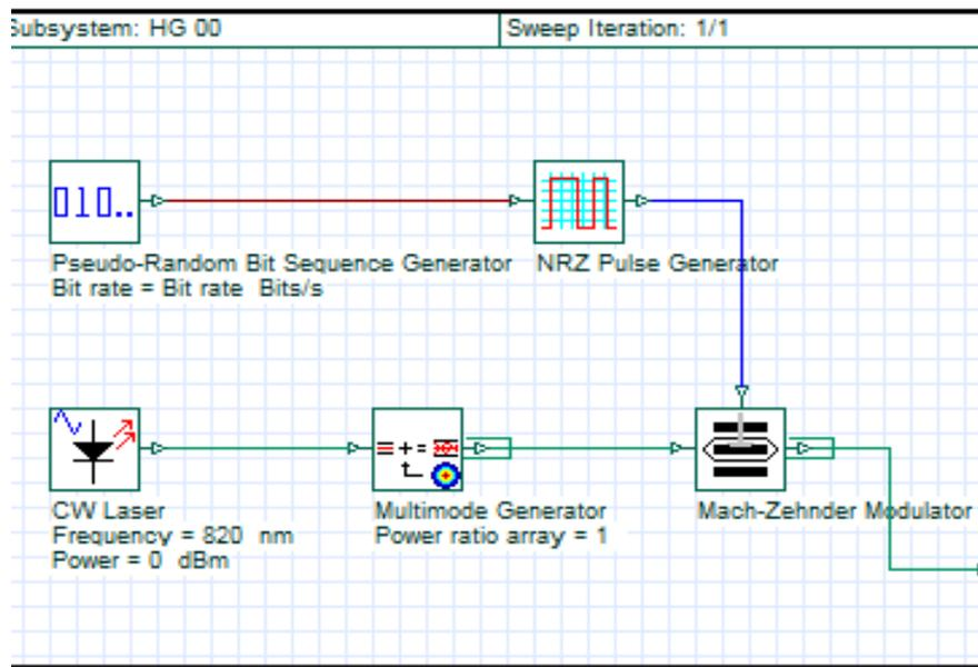
Fig. 4 Data generation of HG00 mode
