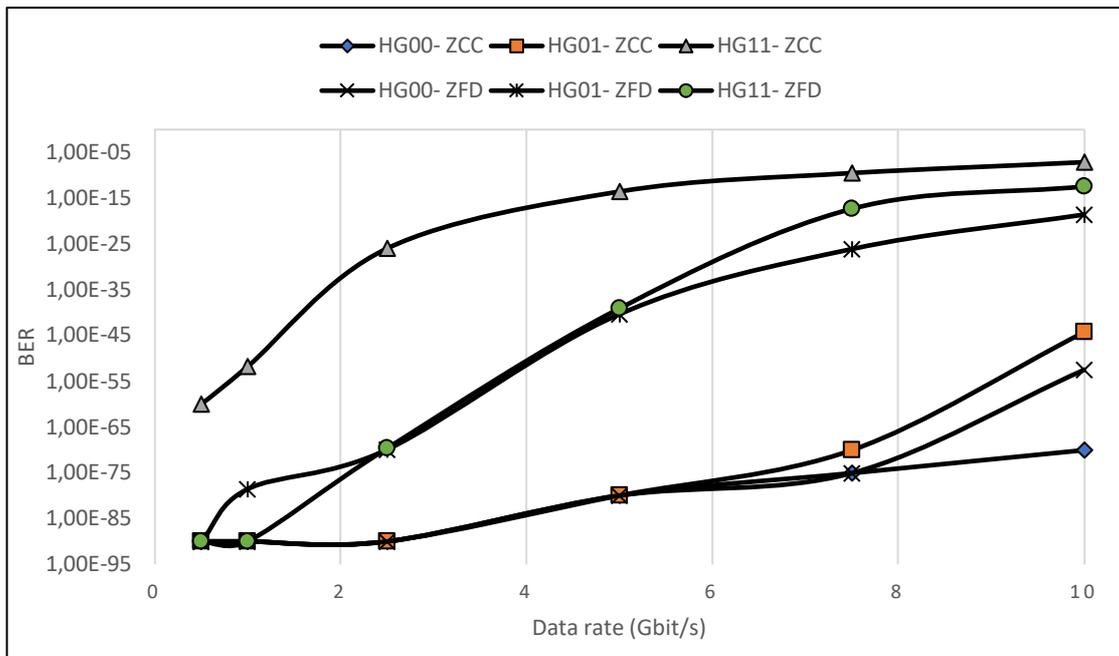
Fig. 7 BER versus data rate
