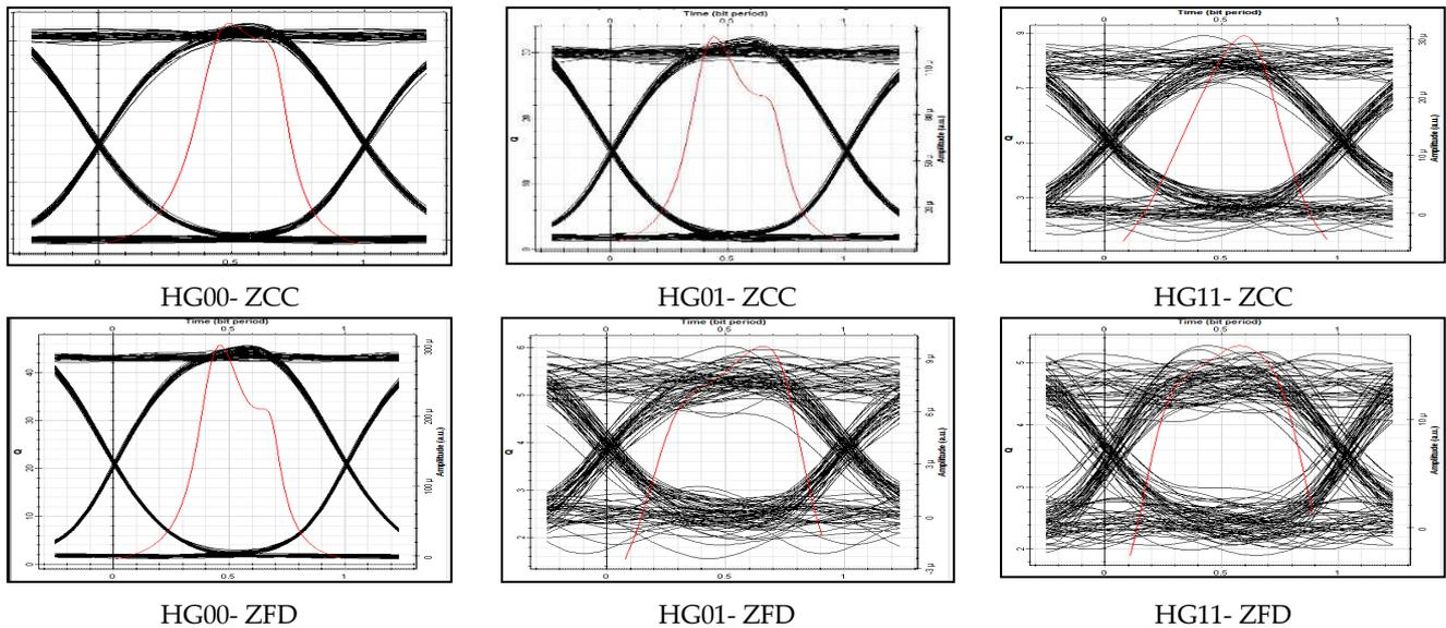
Fig. 6 Eye diagram at 3 km (10 Gbit/s)
