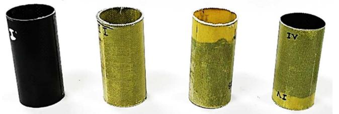
Fig. 2 Moulded tubes ready for crush tests of hybridization schemes of I to IV, from left to right
