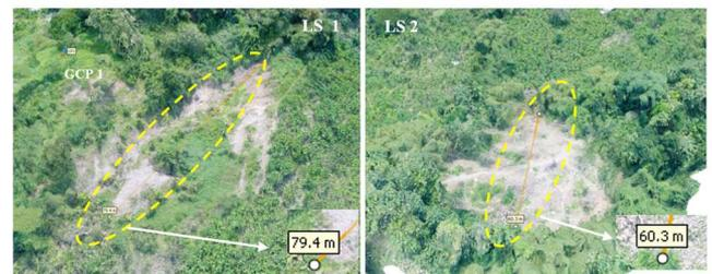
Fig. 11 Landslide Indicated by Ground Movement in LS 1 and LS 2
