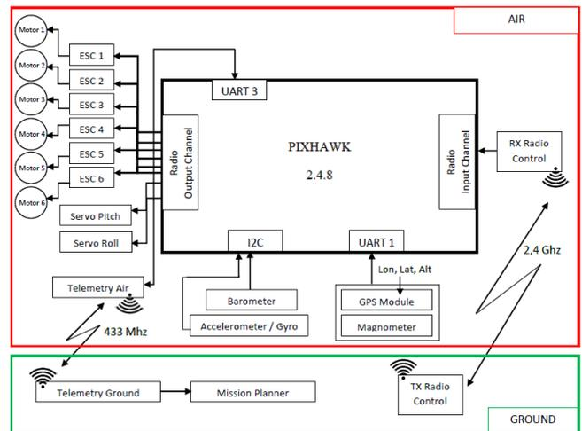
Fig. 1 UAV System Block Diagram
