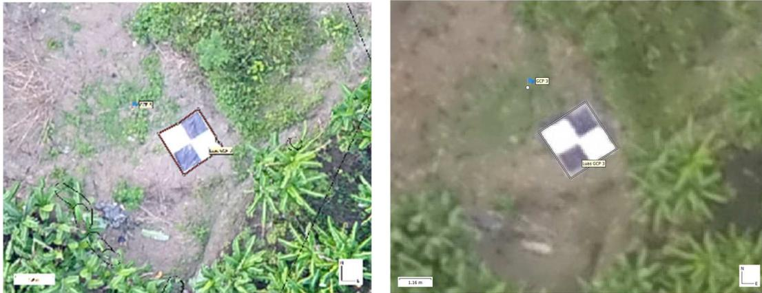
Fig. 8 Results from Polines 01-GD (right) and DJI Phantom 4 Pro (left)
