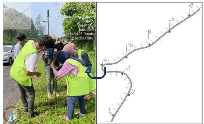
Fig. 6 Collection of CBR Data (Example at point 4)
