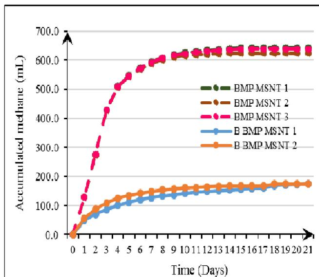
Fig. 3 Cumulative methane production from digesting DMSS; organic content of 0.68
