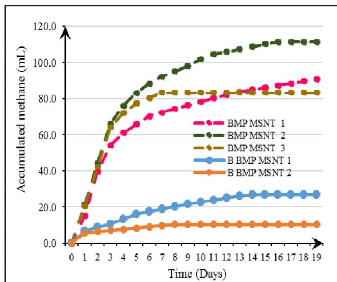
Fig. 2 Cumulative methane production from digesting DMSS; organic content of 0.52
