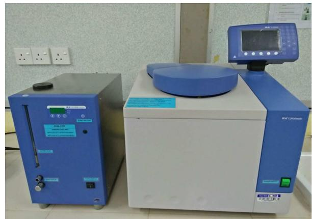
Fig. 2 Bomb Calorimeter C 2000 Basic
