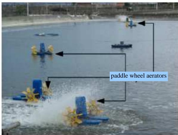
Fig. 9 Aeration system consisting of many paddle wheel aerators operated automatically based on the DO value of the water
