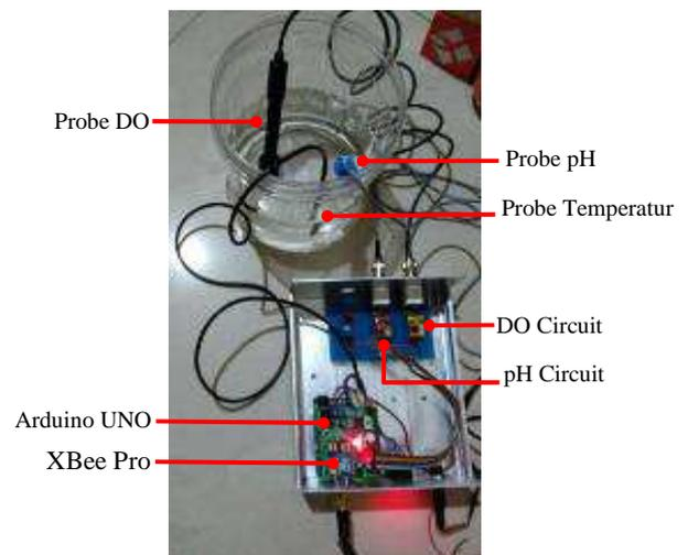
Fig. 3 Block diagram of the sensor module
