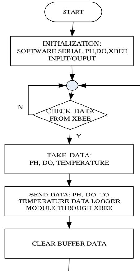
Fig. 2 Flowchart program Arduino Uno
