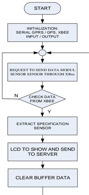
Fig. 5 Flowchart program data logger module
