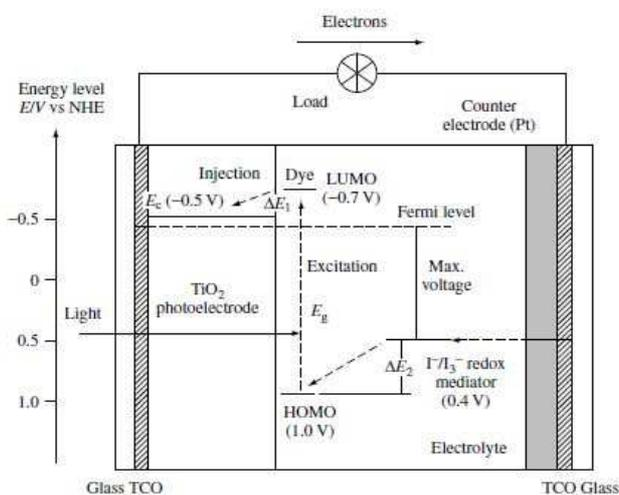
Fig. 2 Schematic energy diagram and operating principle of DSSC
