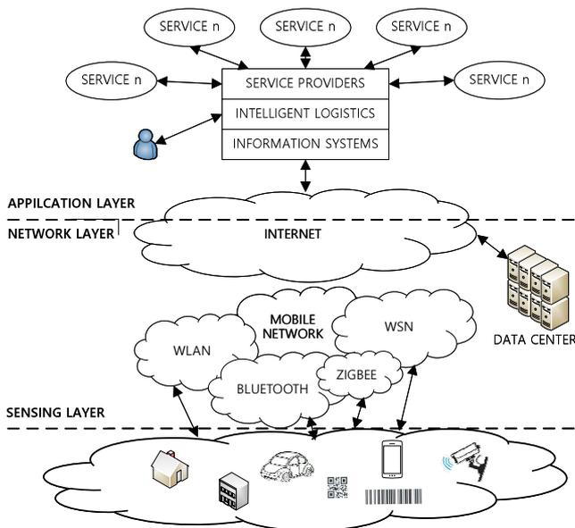
Fig. 1 Basic IoT architecture
