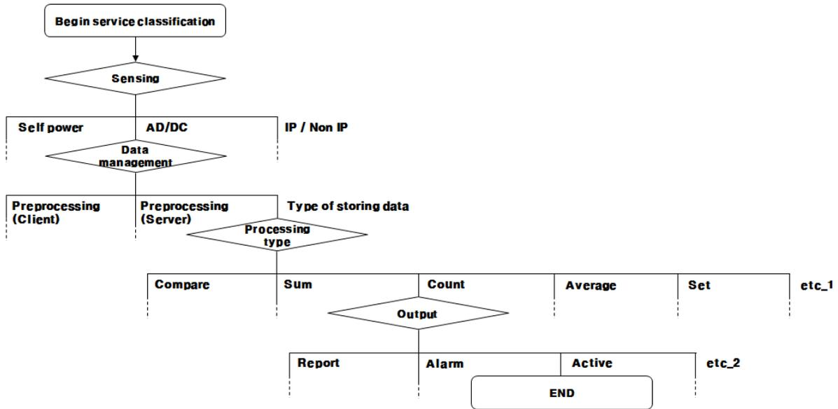
Fig. 4 Example flow of proposed classification algorithm
