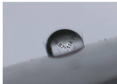
Fig. 8 The contact angle being formed by a water droplet on the surface of a silicone-rubber post-insulator
