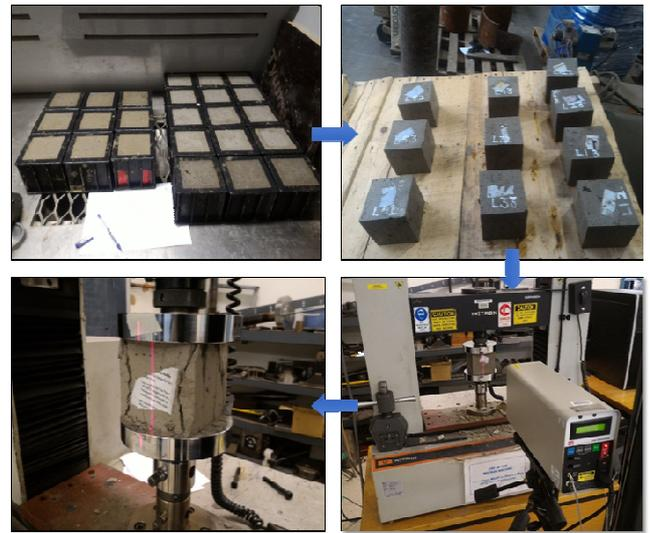
Fig. 2 Schematic of the experimentation, including moulding of composite (top left), curing of samples (top right), testing of samples for geotechnical properties (bottom left and right)
