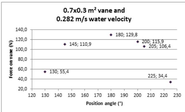
Fig 2. Force on single vane for different vane position angle
