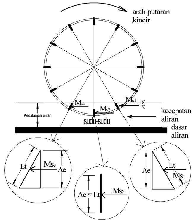
Fig 3. Area of vane toward water flow at different vane position angle
