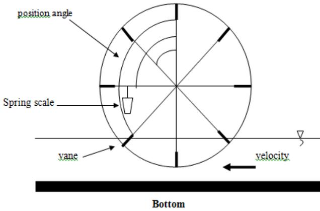
Fig 1. Spring scale use to determine moment of vane force
