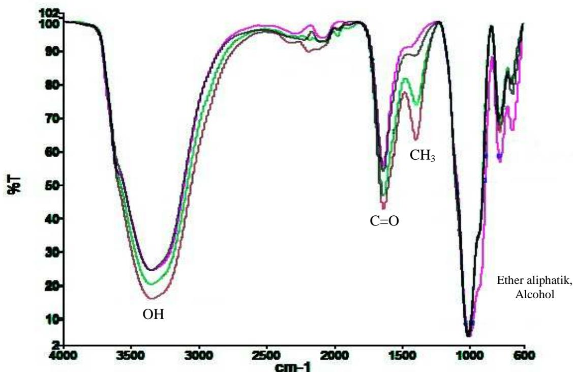
Fig.1. FTIR of powder coal *Sub-bituminous* (purple), 3% of NaOH + powder coal *Sub-bituminous* (blue), 6% of NaOH + powder coal *Sub-bituminous* (green), and 9% of NaOH + powder coal *Sub-bituminous* (red)
