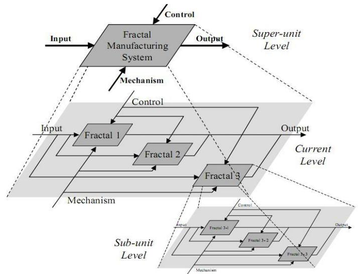
Fig. 2 Conceptual structure of fractal manufacturing system
