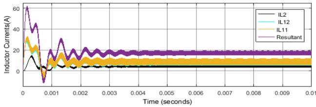
Fig. 25 Inductor currents at each phase and each stage
