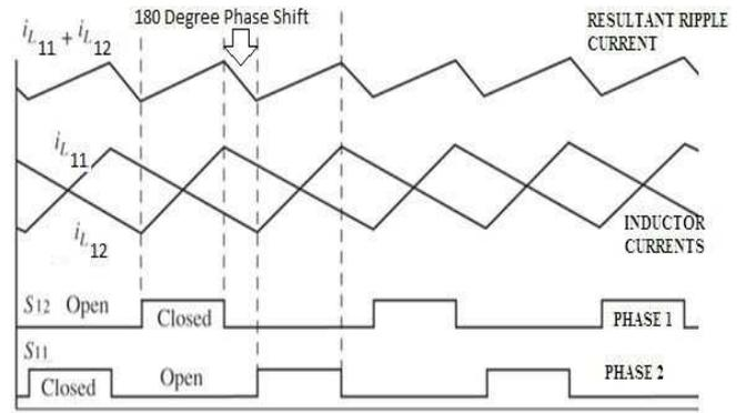
Fig. 2 Dual phase inductor and resultant current
