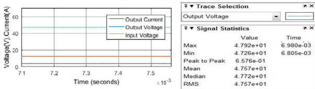
Fig. 9 Enlarged and signal statistics of output voltages
