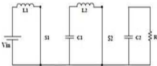
Fig. 4 Both switches ON
