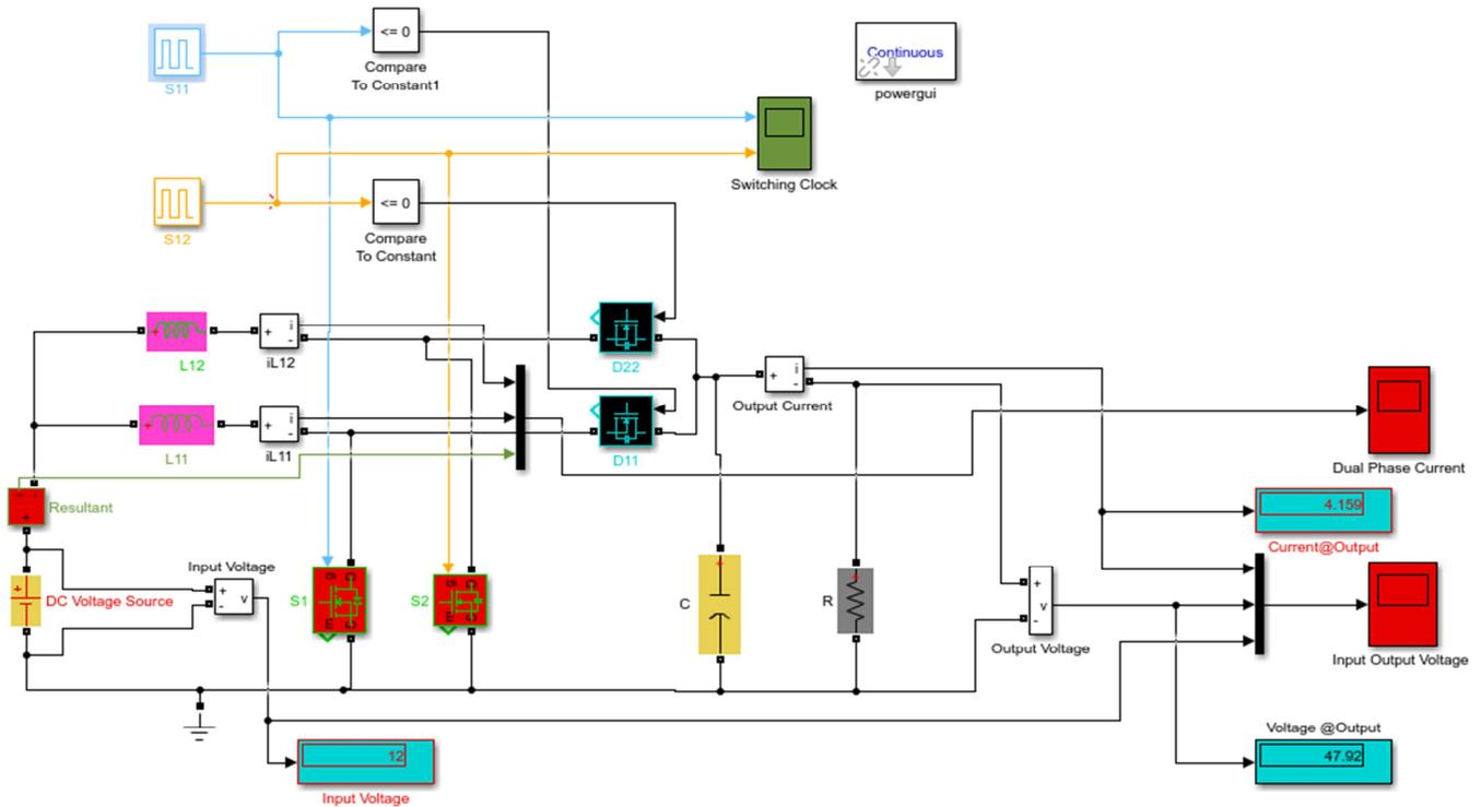
Fig. 7 Simulink Model of Dual Phase Boost Converter
