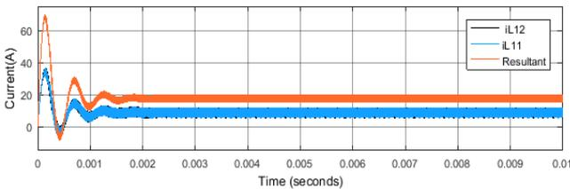
Fig. 10 Individual Phase Inductor current and Resultant
