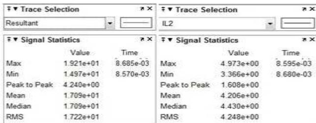
Fig. 27 Signal statistics of Resultant Inductor Current and IL2
