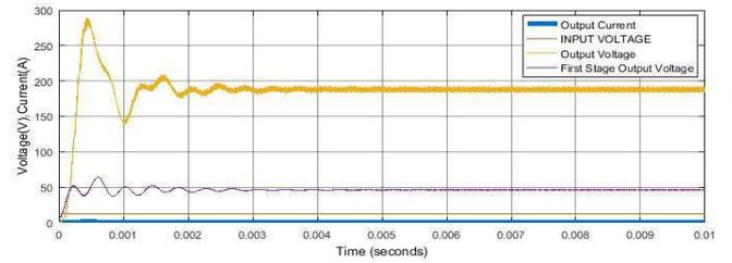
Fig. 21 Voltages at each stage of dual phase dual stage boost converter
