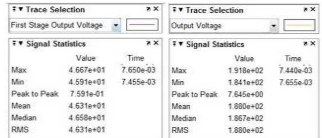
Fig. 23 Signal statistics of first and second stage output voltages
