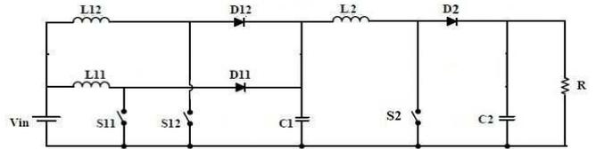
Fig. 6 Dual phase dual stage boost converter
