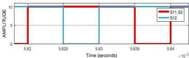
Fig. 28 Switching pulses of three switches S11, S12, S2
