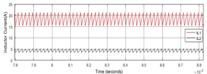
Fig. 18 Enlarged waveforms of inductor current IL1, IL2
