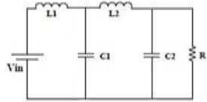
Fig. 5 Both switches OFF
