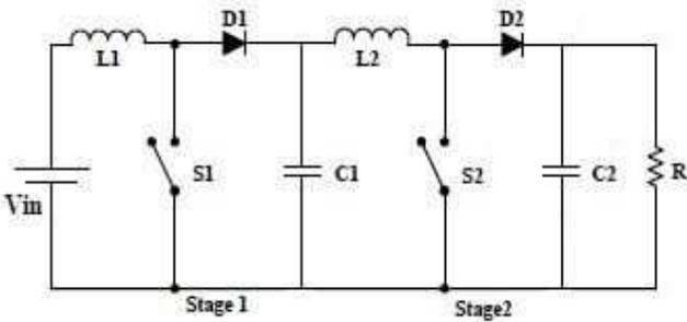
Fig. 3 Dual stage boost converter
