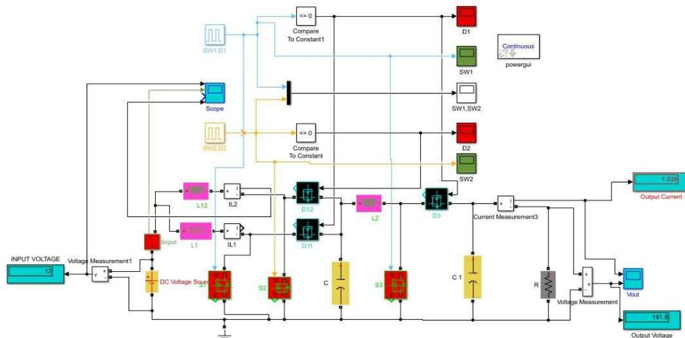
Fig. 24 Simulink model of dual phase dual stage boost converter
