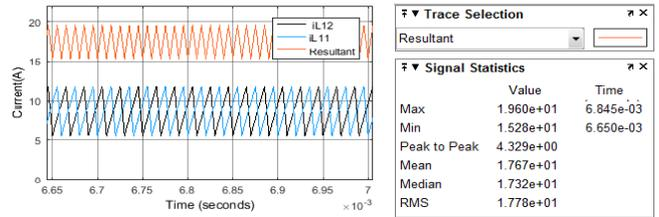
Fig. 11 Enlarged and signal statistics of resultant current
