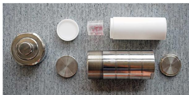
Fig. 4. Autoclave reactor (250 ml)
