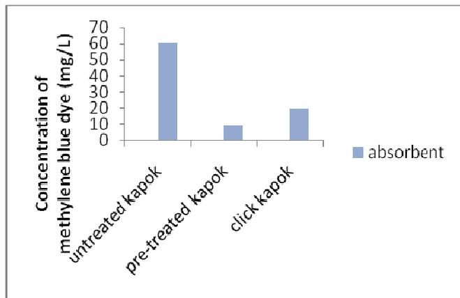
Fig 3 The concentration of methylene blue dye after 24h being immersed with different absorbent
