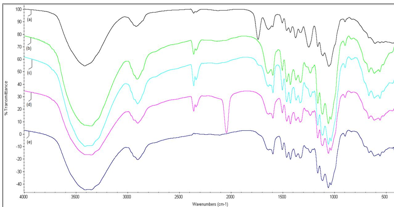
Fig 1 The FTIR result for a) untreated kapok fiber b) pre-treated kapok fiber c) tosylated kapok fiber d) azidated kapok fiber e) click kapok fiber
