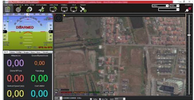
Fig. 9 The Mission Planner software is used to provide the waypoints.
