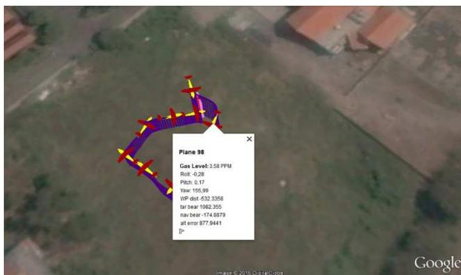
Fig. 15 The result of gas mapping carried out by the quadcopter.
