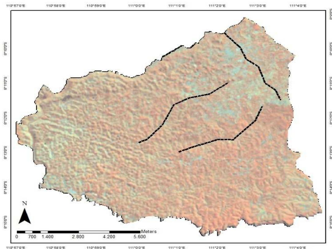
Fig. 2 Color composite result of 567 bands from Landsat 8 image and lineament interpretation (black dotted lines).
