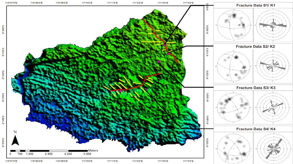
Fig. 5 Joint/fracture data analysis in stereography projection, lineament analysis (red line) and shifting ridge analysis (yellow line) based on SRTM image.
