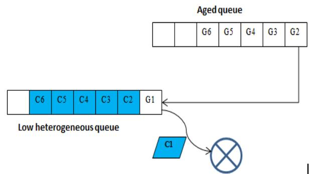
Fig. 4. Inserting G packets into low heterogeneous queue
