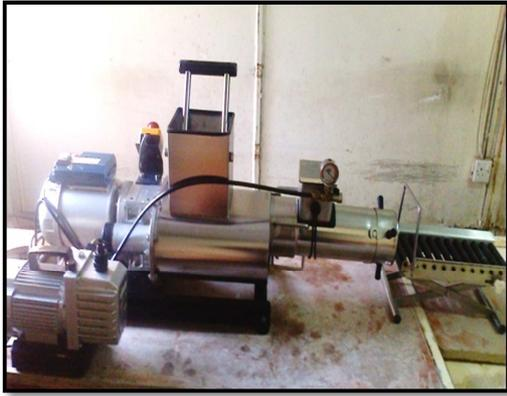
Fig. 3 Laboratory clay extrusion device
