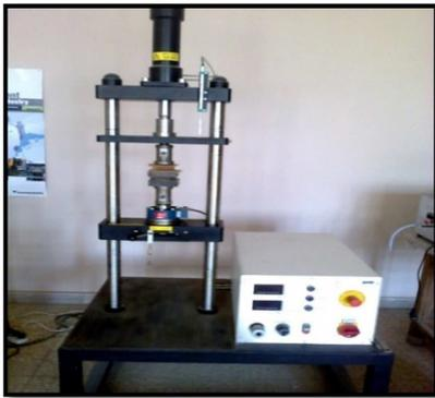
Fig. 6 Compressive strength test machine.
