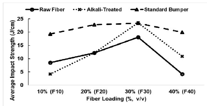
Fig. 2 Impact strength exhibited by the RSF-reinforced composites at various fibre loadings.
