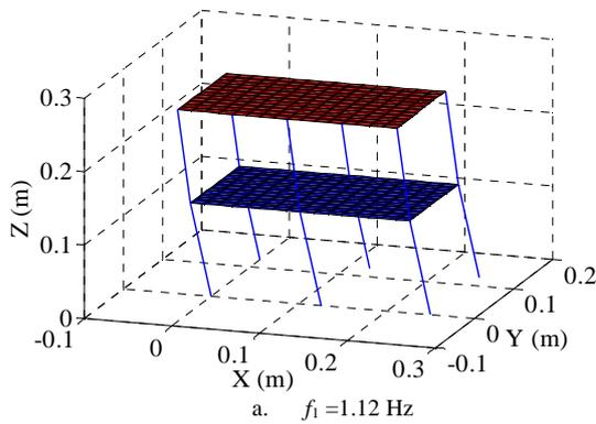
shape relating to the first bending mode on  $x$ - $z$  and  $y$ - $z$  plane, respectively. The natural frequencies of the 1<sup>st</sup> and 2<sup>nd</sup> mode shapes are 1.12 Hz and 1.68 Hz, respectively.
