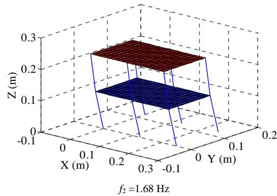
Fig. 4 Two lowest modes of the structure
