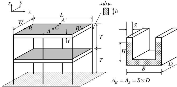
Fig. 2 Scheme of the two-storey building and water tank
