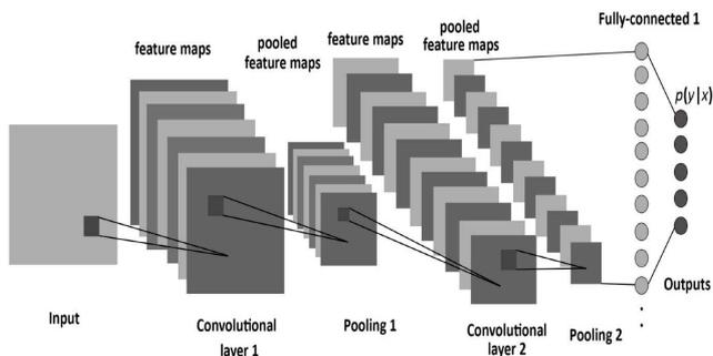
Fig. 6 A basic structure of Convolutional Neural Network (CNN)[104].
