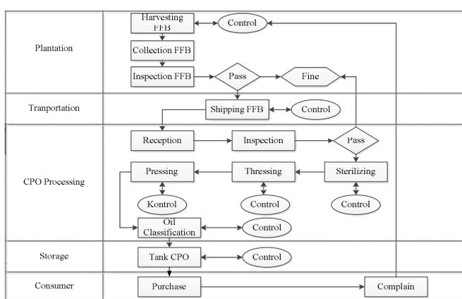
Fig. 4 Production process flow of CPO
