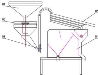
Fig. 10 Schematic diagram of centrifugal breaking and cleaning of cocoa beans with capacity is 80kg/h.
