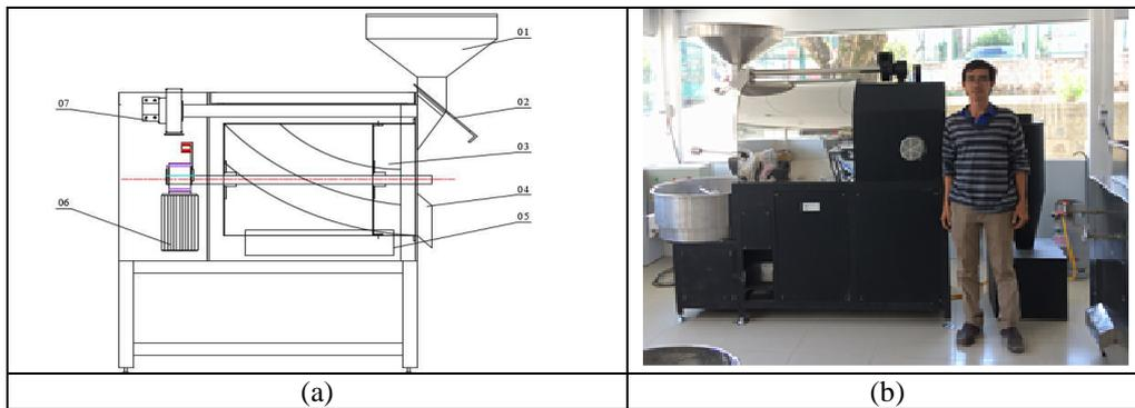
Fig. 6 (a) Roasting machine with the capacity of 10kg / batch working principle diagram. 1. Feed hopper; 2. Beans adjusted supplier; 3. Drum roaster; 4. Roasted bean exit; 5. Infrared gas burner; 6. Engines; 7. Suction fans. (b) Roasting machine with the capacity of 10kg / batch
