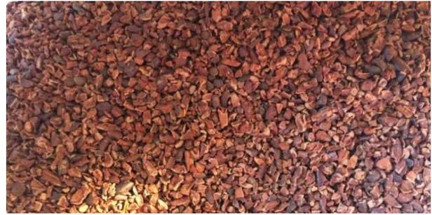
Fig.12 The nibs after breaking and winnowing used centrifugal principle
