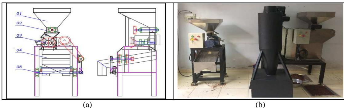
Fig.7 (a) The structure Diagram of the breaker with the principle of grinding 1. Feed hopper; 2. Beans agitator; 3. the breaking part; 4. Screening; 5. Nibs exit door (b) Breaking according to the principle of grinding and cleaning according to the principles of aerodynamics
