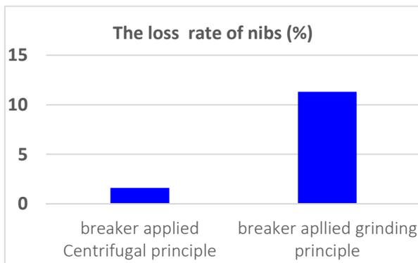
Fig.14 The loss rate of nibs between two principles of breaking and winnowing
