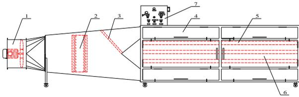
Fig. 5 Dryer used for experiments [11] 1. Fans, 2. Resistivity, 3. Wind wing, 4. Drainage door, 5. Drying tray, 6. Drying door, 7. Electric control cabinet.
