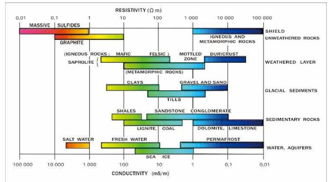
Fig. 3 The range of resistivity and conductivity value of the materials of the earth, water, soil, minerals and rocks [14]
