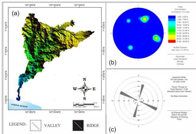
Fig. 9 (a) The geological structure analyzes of the study area in the form of lineament of valley and ridge on SRTM-DEM image with the general direction of NW-SE and NE-SW, (b) and (c) joints analysis use DIP program with the general direction of NW-SE and NE-SW.
