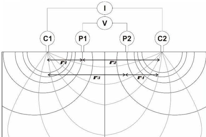
Fig. 4 Electrode Schlumberger configuration geoelectric method
