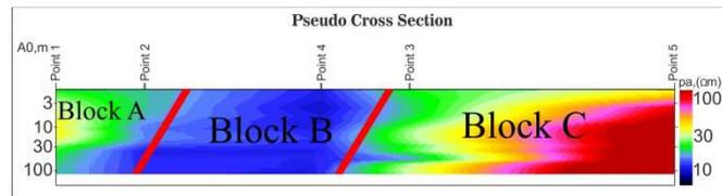
Fig. 6 The 2D false colour cross section of geoelectric measurement, GL1-GL 5 trajectory with height of 195 to 925 meters a.s.l, depth of up to about 120 meters and resistivity values of 6 to 450  $\Omega$  meters in the Cilaki drainage basin
